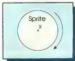
A two dimensional object like a sprite can be rotated only on its center axis. You can however use multiple objects to create an animation sequence that looks like rotation.
